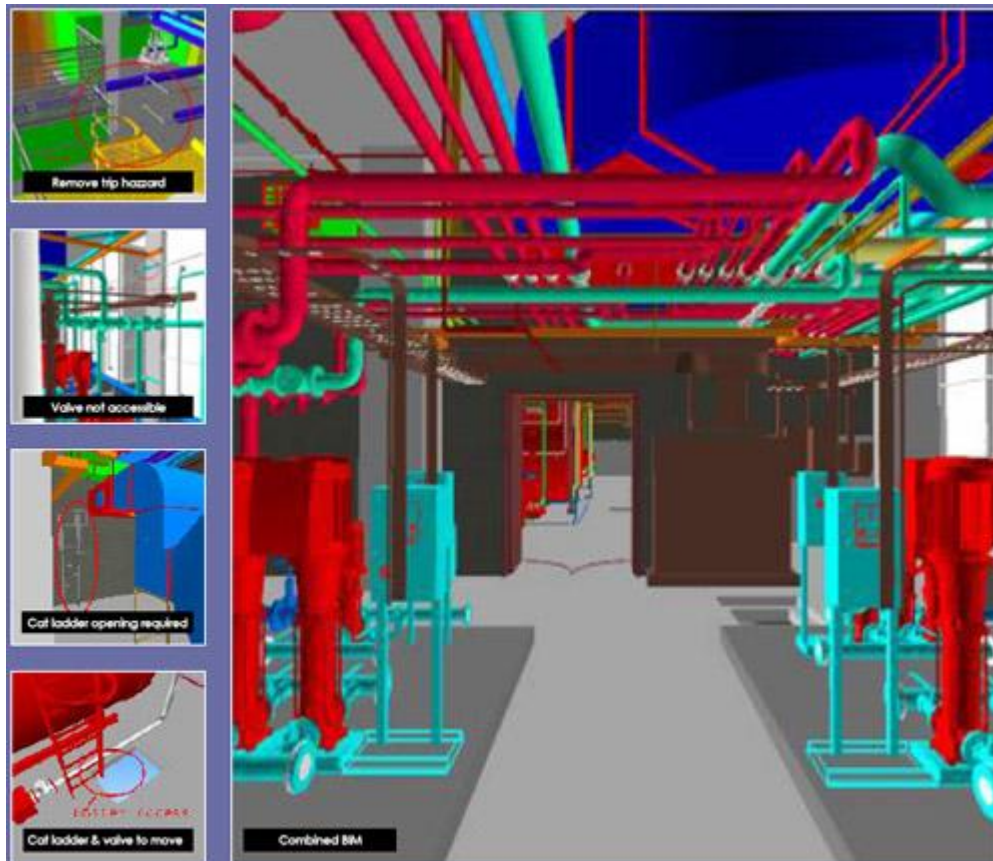
Figure 2. Some of the constructability issues detected by combining the individual disciplinary models in Navisworks. (Courtesy: HOK and Skanska)
